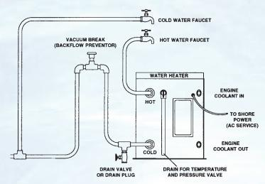
The "1700 Series" water heater provides hot water for galley and shower. Dense foam insulation provides better and longer heat retention than traditional fiberglass. The tank itself is protected by a 75 PSI T& P (temperature and pressure) relief valve. The cylindrical design of the tank enables it to withstand more pressure than a cube shaped tank.
