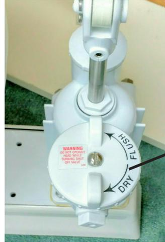
Position for intake of water and discharge of bowl contents
